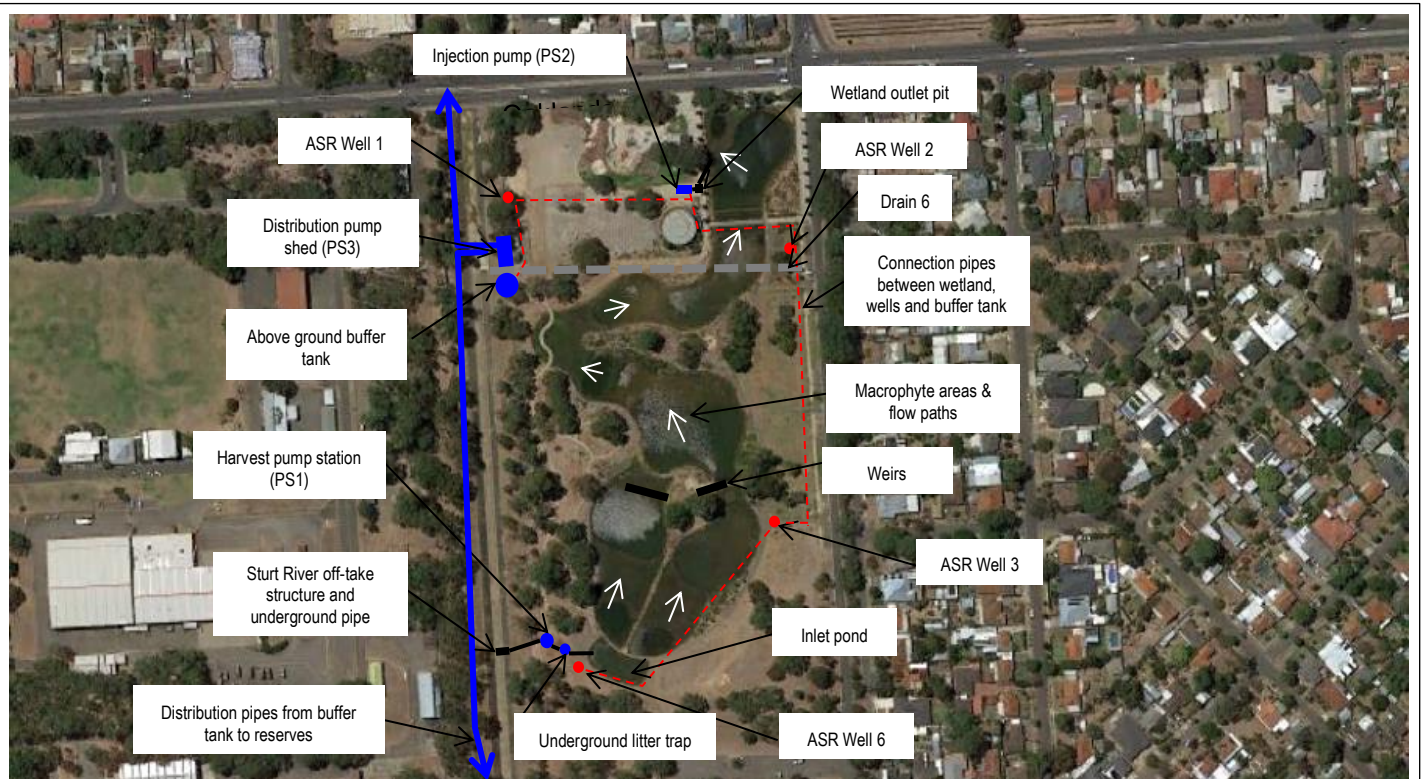
Figure 1 Oaklands stormwater harvest and re-use project
