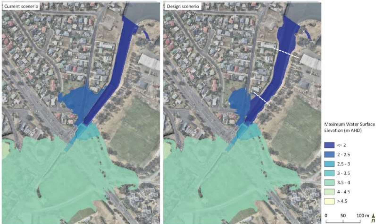
Water Surface Elevation (1% AEP Climate change) – before (L), after (R) Supplied by Alluvium
